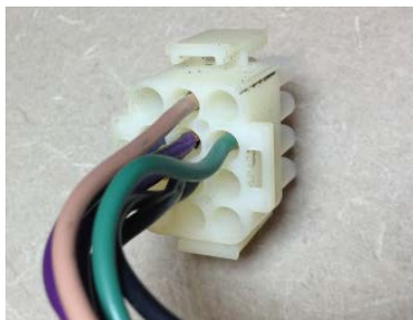
Insert tan engine temp wire in position 2
