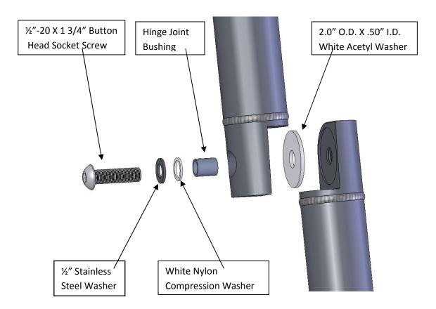
NOTE: The ½" Stainless Steel washer should be assembled to the outside of the White Nylon Compression Washer. This allows the White Nylon Compression Washer to be trapped and compressed into the hinge counter bore. Failure to assemble the Hinge Joints in this way will cause failure of the White Nylon Compression Washer; this may possibly reduce the performance of the Tower shortening the life of the hinge joint.
