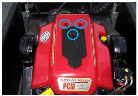
Unscrew the 3 plastic nuts from the engine cover with the 14mm socket and remove cover
