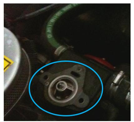
Replace the Thermostat and Gasket.
