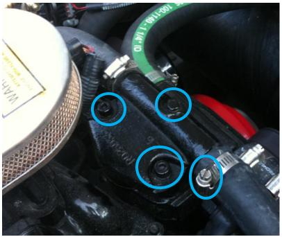
With the 6mm Hex and 10mm socket, remove the bolts With the screw driver loosen the hose clamp and then remove the hose only from the one side. You do not have to remove the hose on the opposite side.
