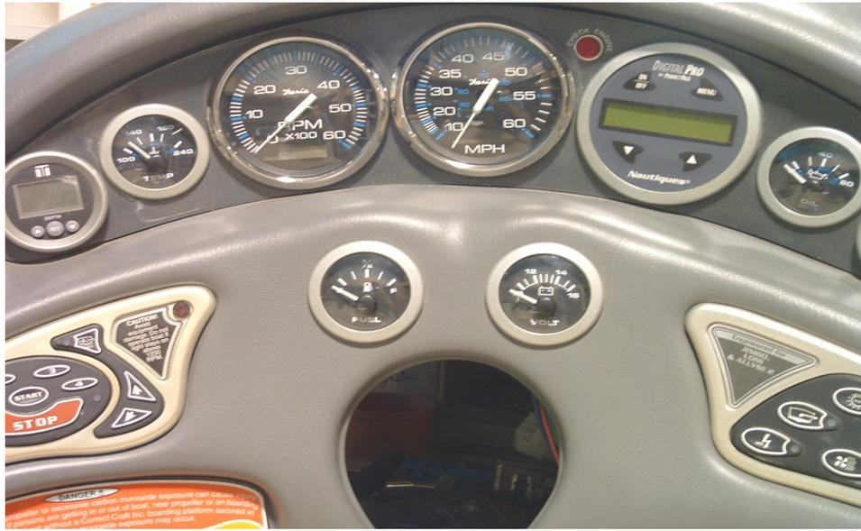
The following are instructions on how to remove the Teleflex MPH and RMP gauges and replace them with the Faria MPH and RPM analog gauges.
