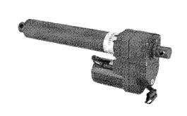
Warner Linear Linear Actuator: 12V DC Input Volt, 2800 lb Load Capacity, 6 in Stroke Lg, 14 in Retracted Lg, 25 A Current
